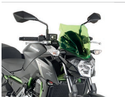
KA4117GR Kawasaki Z650 (17 → 18) Specific "LIME" screen 28 x 33 cm (H x W) →NEW
